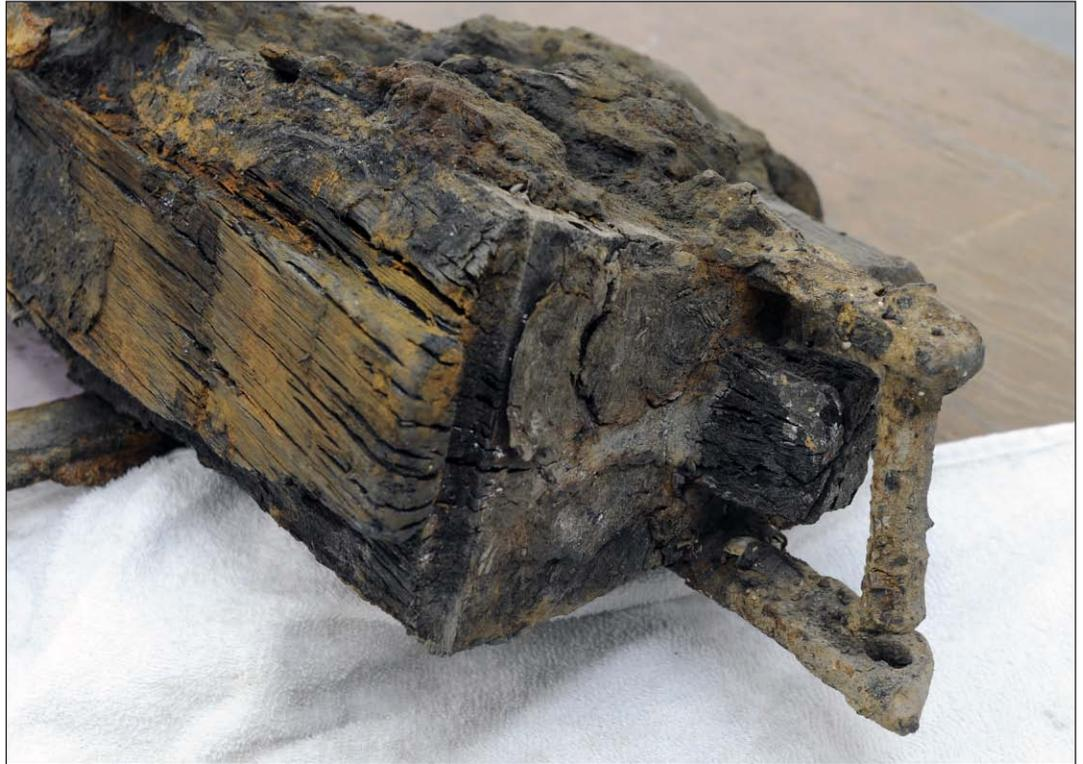
Bottom of sternpost (ST2), which attached to the keel with a projecting wood tenon and iron stirrup. The forward face is to the left of the photograph. Photograph by Drew Fulton
