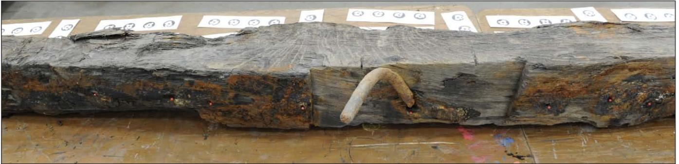
Frame FNFS 23-0 showing a mis-hit iron pin in center. Two marks on aft face of frame **A** correspond to location of keel. Photograph by Drew Fulton
